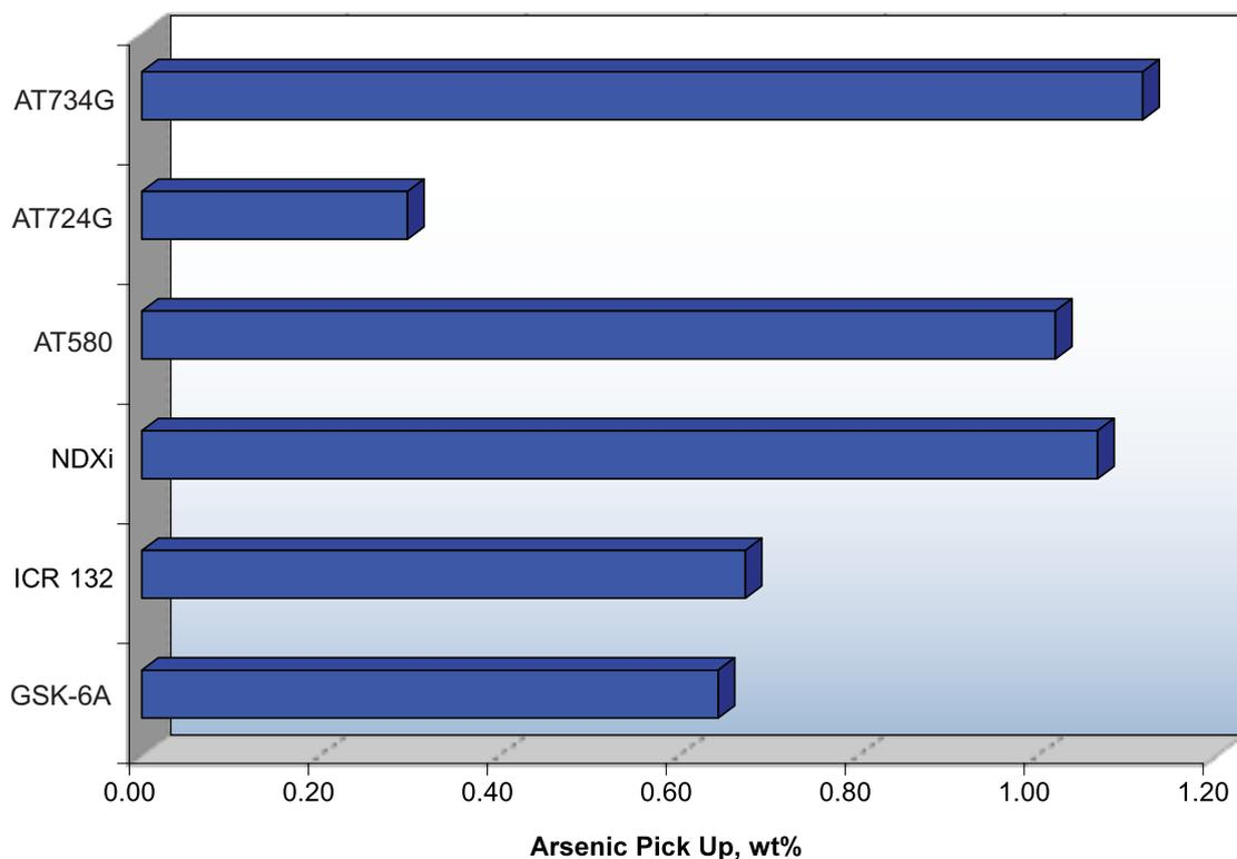
Figure 10 summarizes some results from a catalyst basket where several ART catalysts were evaluated along with AT734G. AT734G picks up about four times more arsenic compared to AT724G, and even picks up more than some high Ni catalysts like NDXi and AT580.
