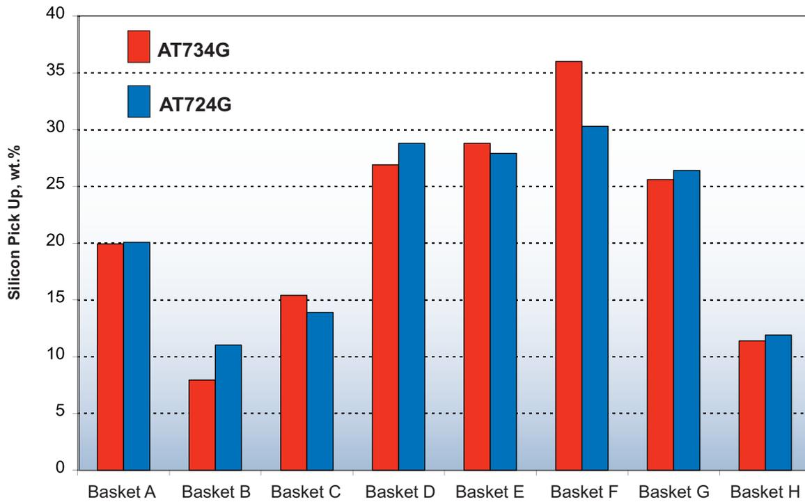
These baskets were installed in coker naphtha units as well as diesel units which suffer from Si poisoning. The data show that the Si pickup of AT734G is on average the same as the Si pickup of AT724G. Notice a few basket samples show extremely high Si pickup, in excess of 25 wt.% Si. These were installed in diesel units and experienced much higher temperatures than some of the baskets showing lower Si values.
