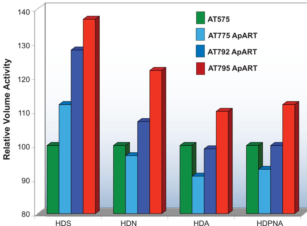
refiners the choice between increasing cycle life or processing more difficult feeds. Figure 14 shows the advantage of using the new system over previous ApART systems with AT575.
