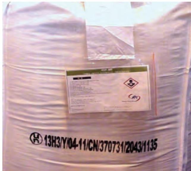
FIGURE 4: UN Approved Catalyst Bags with Appropriate Labeling
